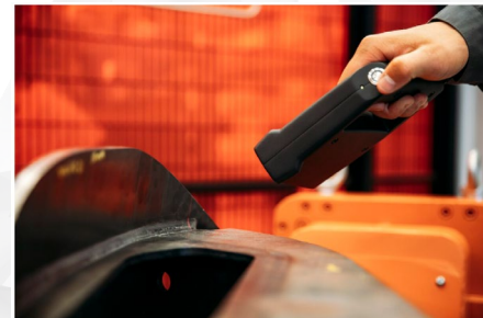
Handheld weld quality scanner – Wintaria FLEX
